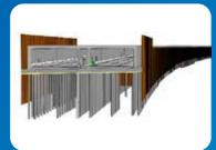
Parametric design involves automating digital design processes through algorithms and computer programming. Thanks to this, the design of a single segment could be automatically reproduced along the entire length of the tunnel, which reduced the risk of errors and saved the engineers time to study alternative design solutions.
